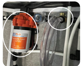
PUMP & 3-WAY VALVE FIGURE C
